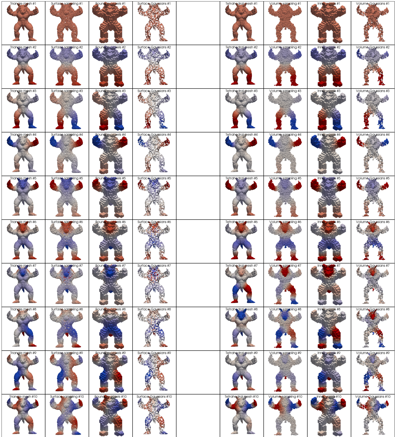
Figure 10. First 10 eigenvectors on the Armadillo, treated as a surface on the left and as a volume on the right. From left to right, the shape is encoded as a triangle mesh, a point cloud sampled uniformly at random, a voxel grid, a Gaussian mixture; a tetrahedral mesh, a point cloud, a binary mask and a Gaussian mixture. Figure 3 corresponds to the last row.
