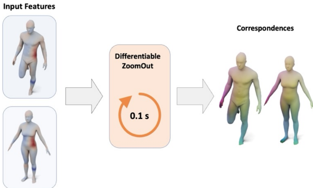
Figure 7.1: Our method takes a set of point features as input, which can be learned and uses a differentiable version of the ZoomOut algorithm to produce correspondences. Due to its light memory cost and attractive processing time this can be used while training a network, or when running the network on very dense meshes.
